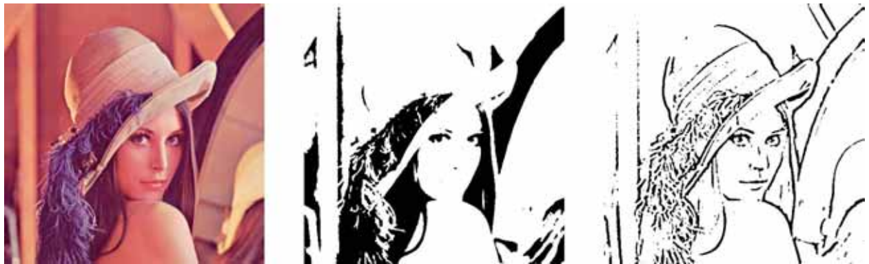
Fig. 6. Thresholding. The input image (left) is converted to the black-and-white thresholding image (center) and adaptive thresholding image (right).
