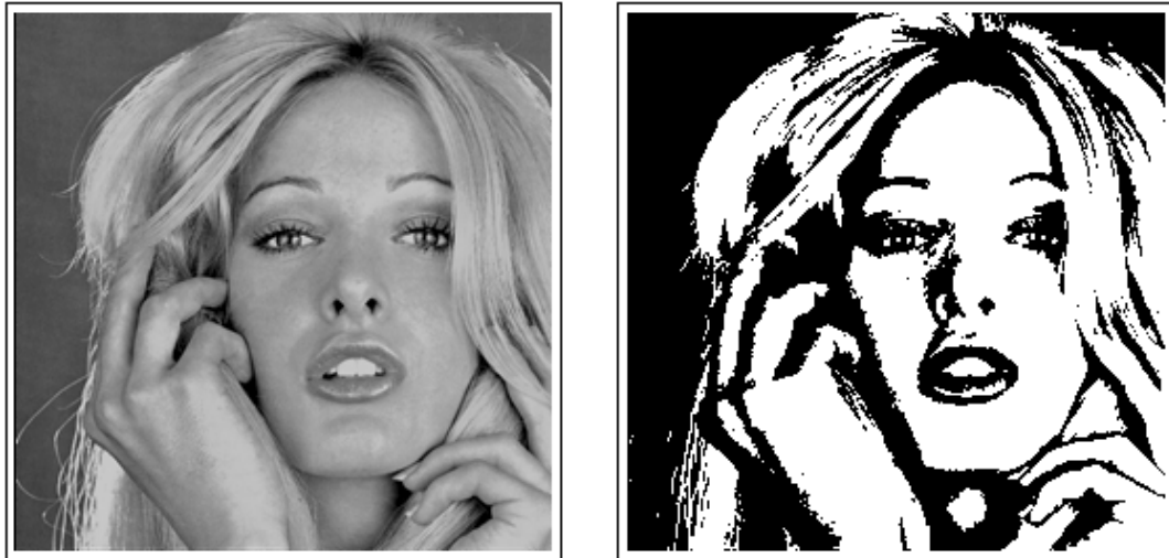
Fig. 11. Thresholding CNN. The woman’s grayscale image (left) is converted to the black-and-white threshold image (right). The threshold z^* is set to 0.1.
