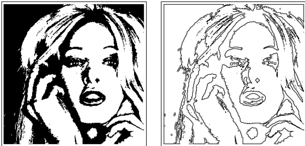
Fig. 12. Edge detection CNN. The threshold image (left) is converted to the edge image (right).
