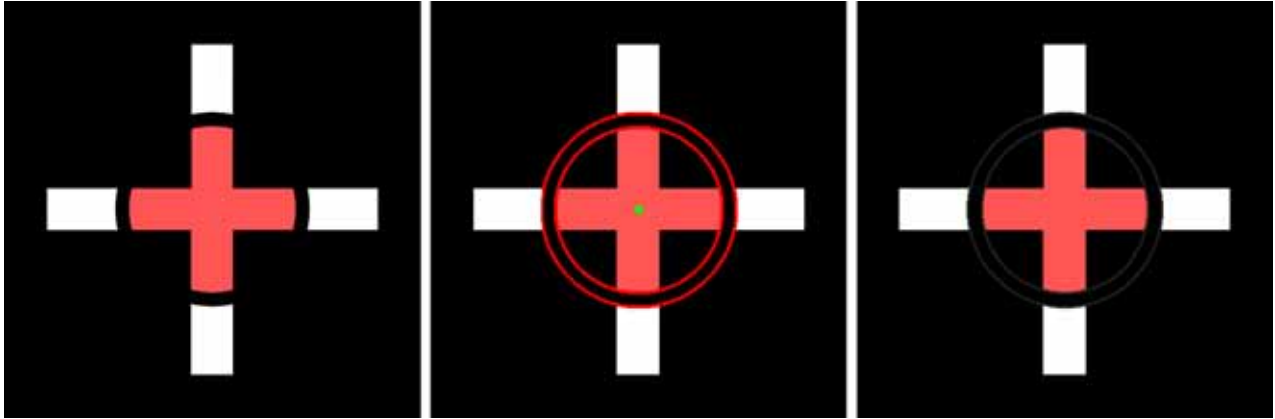
Fig. 39. Neon color spreading illusion image with a black ring. The cvHoughCircles detect two illusory circles from the illusory image (left). Their centers and circles are painted in green and red, respectively (center). The cvCircle emphasizes the black ring (right) by gray lines.
