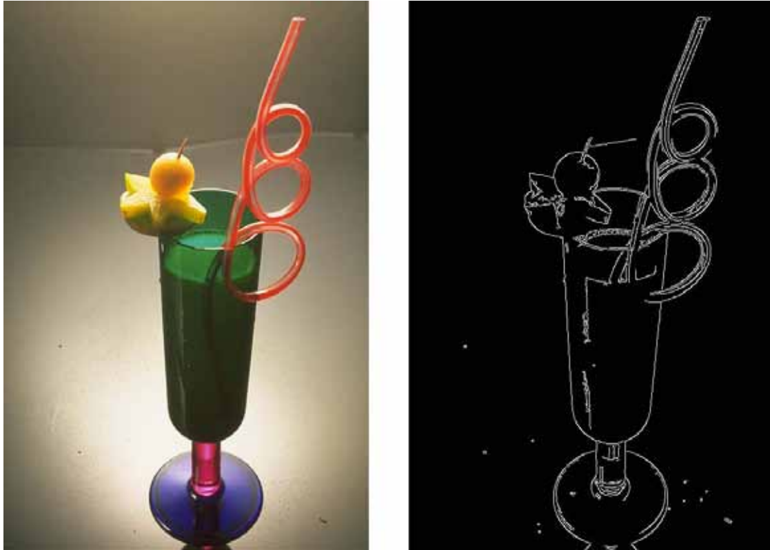
Fig. 7. Canny edge detector. The input image (left) is converted to a black and white image with edges (right).
