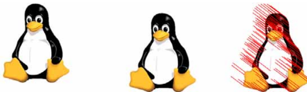
Fig. 9. Optical flow. The motion of image is marked by red lines (right). It is calculated for two input images (left and center), which are included in the OpenCV’s web reference manual.
