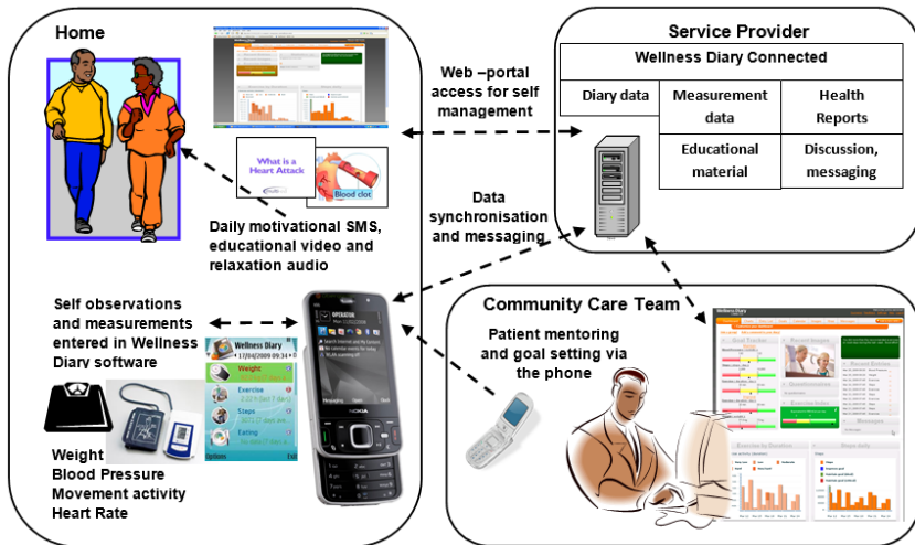
Figure 1. An illustration of the CAP CR program. The mobile phone acts as the communication medium through which a mentor provides mentoring and goal setting, daily motivational messages, educational videos and relaxation audio are sent, and self-observations and measurements are entered to a health diary application.
