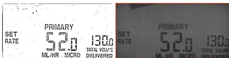
Figure 1. The image files, saved as logs, showed that nurse correctly set the pumping rate to 52 cc/hr.
