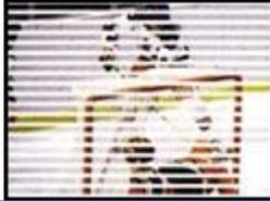
All odd numbered lines are scanned on the screen in 1/60th of a second
