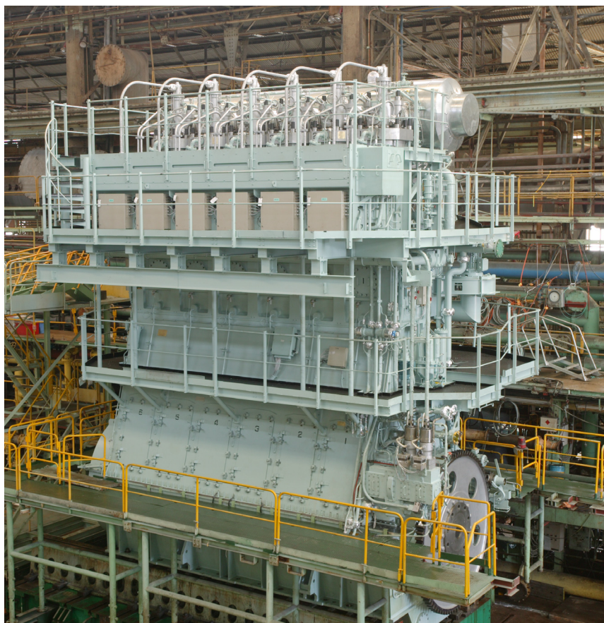
Fig. 2: The first six-cylinder Wärtsilä 6RT-flex50 marine diesel engine. It has a maximum continuous power of 9960 kW at 124 rpm, and measures about 9.4 m in overall height, and 7.1 m in overall length. [05#186]
