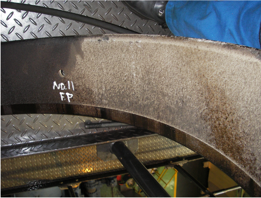
Fig. 7: The Anti-Polishing Ring (APR) for RTA96C and RT-flex96C engines has a revised geometry with two edges to clean the piston top land during both the up and down strokes of the piston. [05#241]
