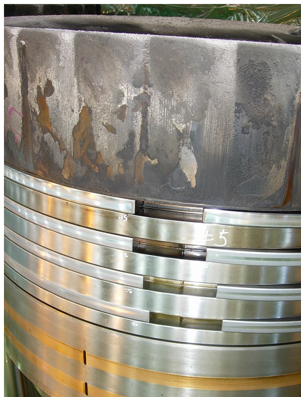
Fig. 6: Piston of an RTA96C engine after testing at 110 per cent load. This piston is according to the latest design standard with chromium-ceramic rings in all grooves and with two bronze rubbing bands in the short skirt. [05#240]
