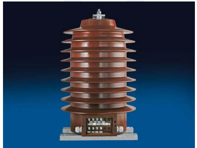
Outdoor voltage transformer with characteristic shields to extend the creepage distance
